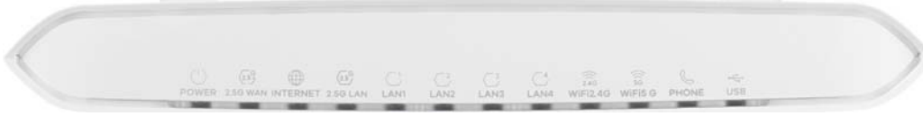
Figure 7 LED Indicators (AX7501-B0 / PX7501-B0)
