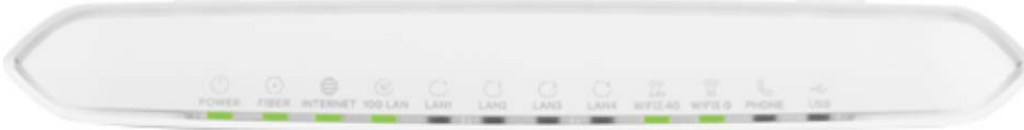
Figure 7 LED Indicators (AX7501-B0 / PX7501-B0)
